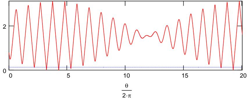
A proper calculation of the fraction of time that satellite is within range of target would integrate the function  $\text{if}(A(\theta) < \alpha, 1, 0)$  from  $\theta = 0$  to  $2\pi m$ , where  $m$  is the number of unique orbits:
