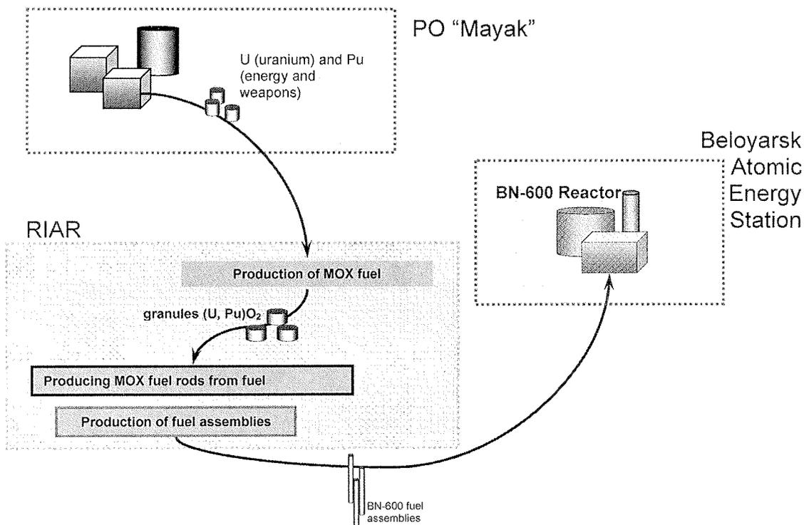
Figure 4 Planned fueling of the BN-600 reactor using highly enriched uranium and separated plutonium already in storage.
