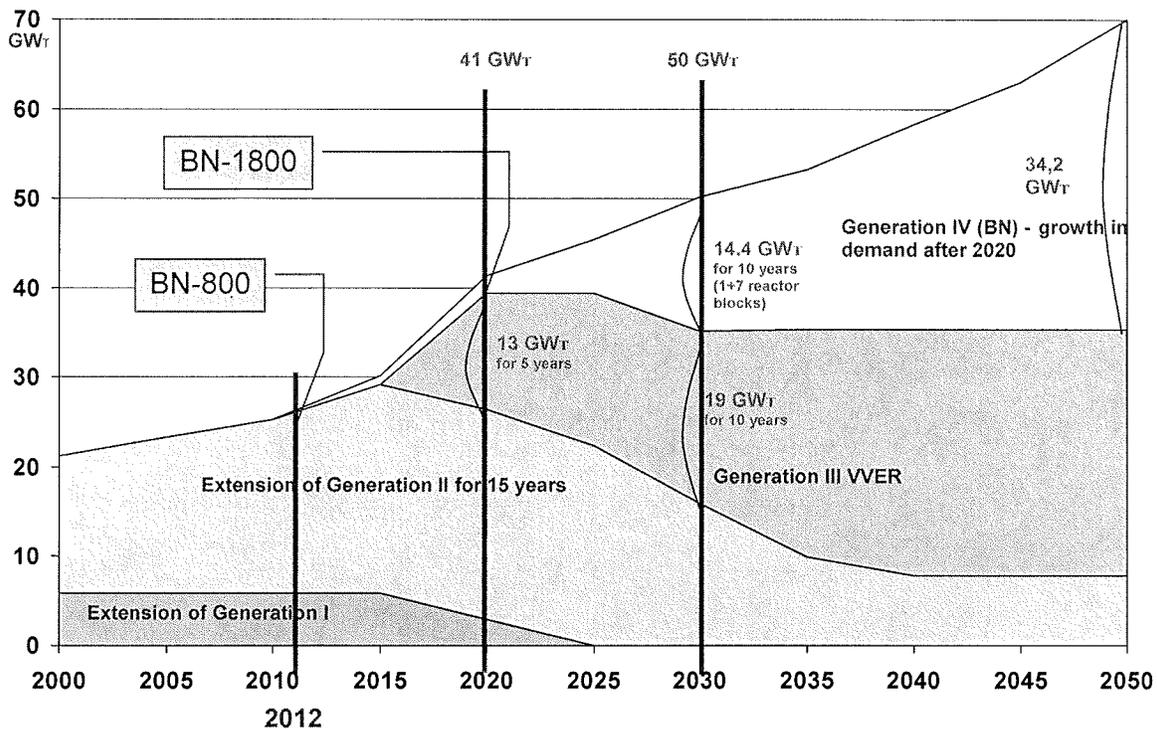
Figure 3 Planned contributions of different reactor types to nuclear power generation in the Russian Federation through 2050.<sup>3</sup>
