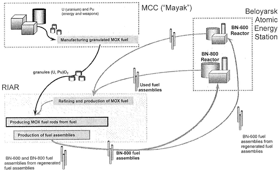
Figure 5 Planned closed fuel cycles involving the BN-600 and BN-800 reactors.
