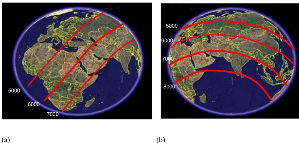
FIGURE 4-5 Sample great circle ranges (nmi) from (a) Kennedy Space Center, Florida, and (b) Vandenberg Air Force Base, California, illustrating the need for 6,500 to 7,000 nmi to reach most parts of the world for a continental United States-based system. Overflight restrictions can result in significantly longer range requirements, since the vehicle may be required to travel the long way around the globe.
