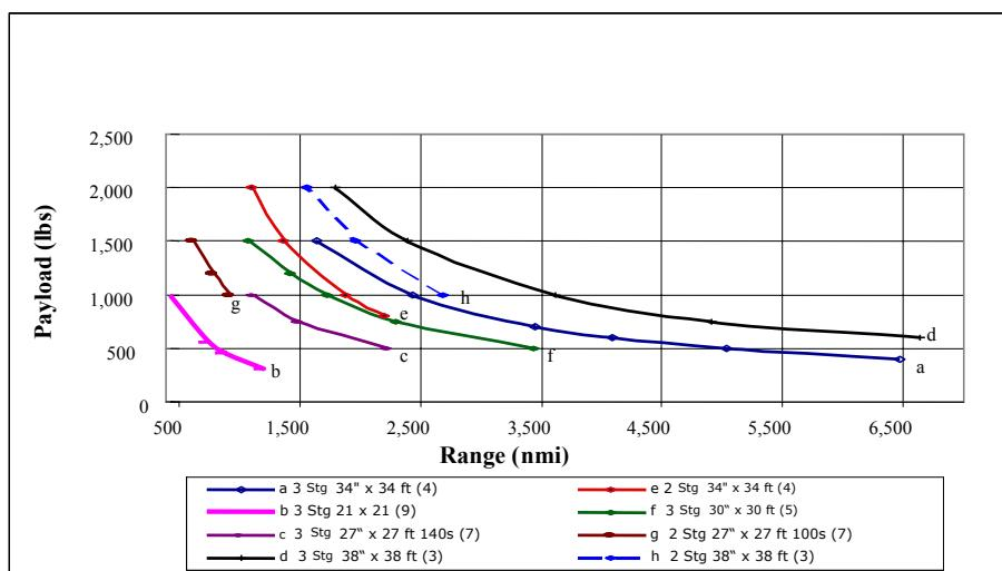
FIGURE 4-12 Payload versus ballistic range capability for notional two- and three-stage Submarine-Launched Global Strike Missile (SLGSM) configurations. All vehicles are constrained to a length-to-diameter ratio of 12. The number in parentheses indicates the number of missiles that can fit in a single launch tube of a nuclear-powered guided missile submarine.
