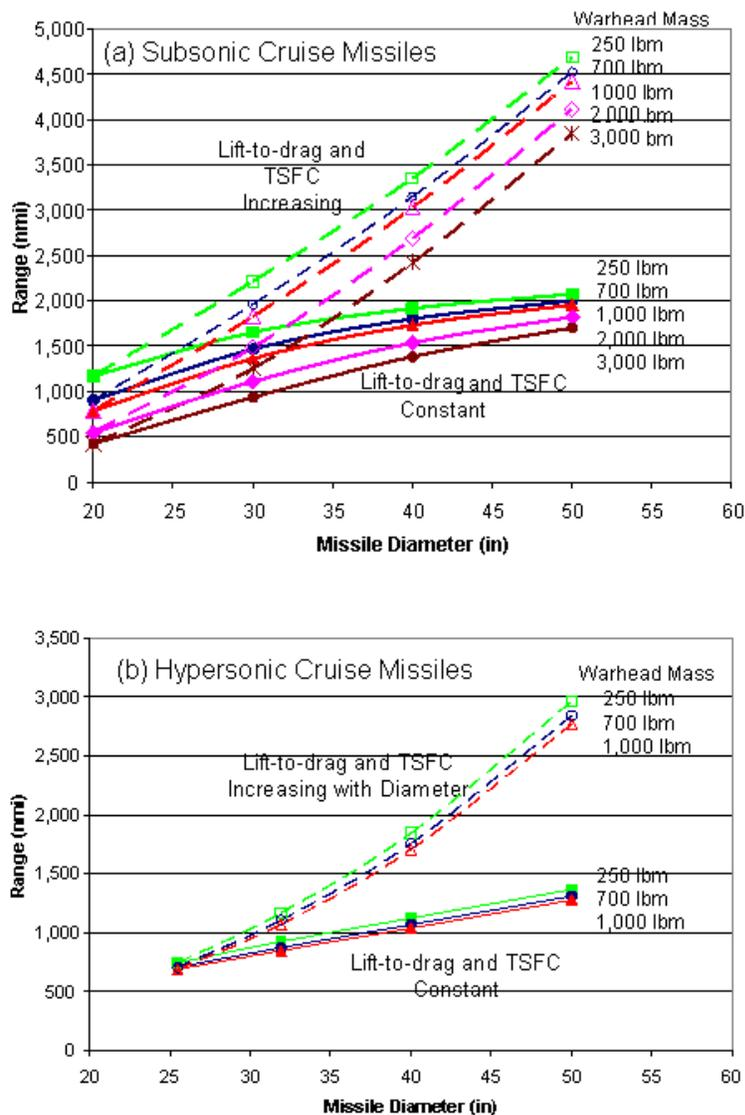
FIGURE 4-14 The impact of missile diameter and payload on range of notional (a) subsonic and (b) hypersonic cruise missiles. The solid curves are based on flight- or laboratory-demonstrated aerodynamic and propulsion technology. The dashed curves illustrate the potential performance improvements that result from potential aerodynamic and propulsion efficiency gains. NOTE: TSFC, thrust specific fuel consumption.
