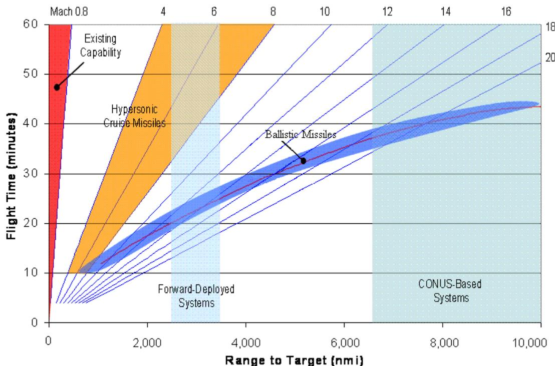
FIGURE 4-7 Flight time versus range for existing subsonic systems, proposed hypersonic cruise missiles, and ballistic missiles. Overlaid are lines of average Mach number, defined as the ratio of block speed (range divided by flight time) to the sound speed at 390 degrees Rankin. For continental United States (CONUS)-based systems, only ballistic missiles are capable of meeting a 1-hour time line. For forward-deployed systems, hypersonic cruise missiles are candidates.
