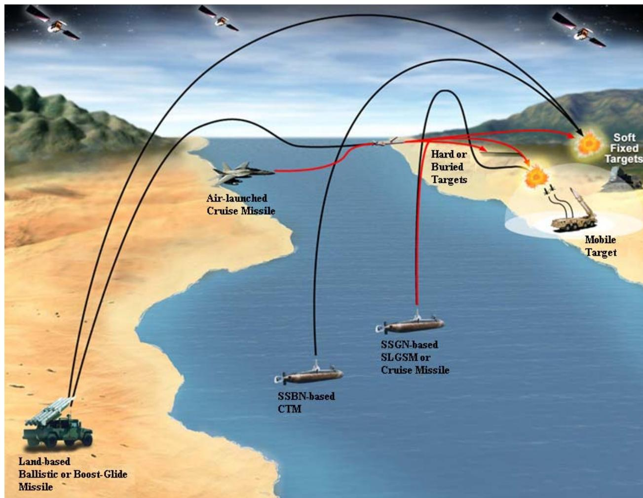
FIGURE 4-1 Candidate concepts for conventional prompt global strike include ballistic missiles, boost-glide vehicles, and hypersonic cruise missiles. The range of these concepts varies from 1,000 to 3,000 nmi for forward-deployed systems to more than 10,000 nmi for land-based systems. Options are being investigated to attack a range of targets from soft to hard to mobile. NOTE: Acronyms are defined in Appendix A.
