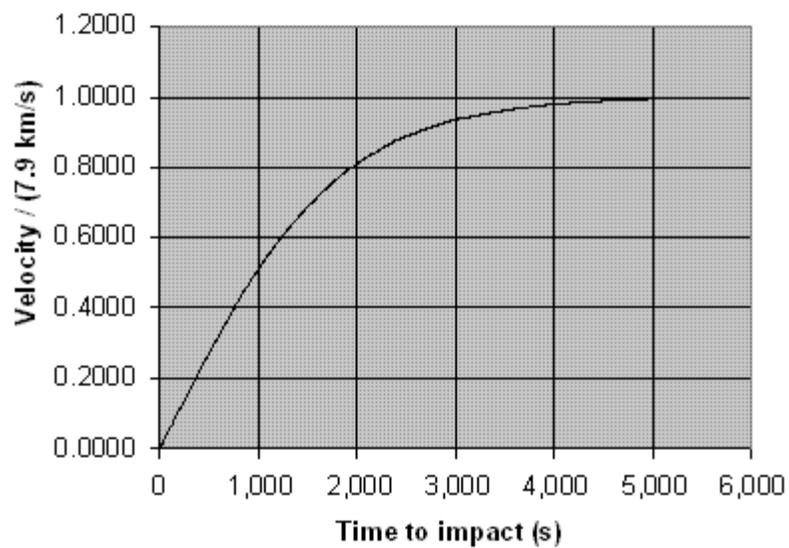
FIGURE G-4 Velocity versus time for pure glide (Columns C versus B of Table G-1).
