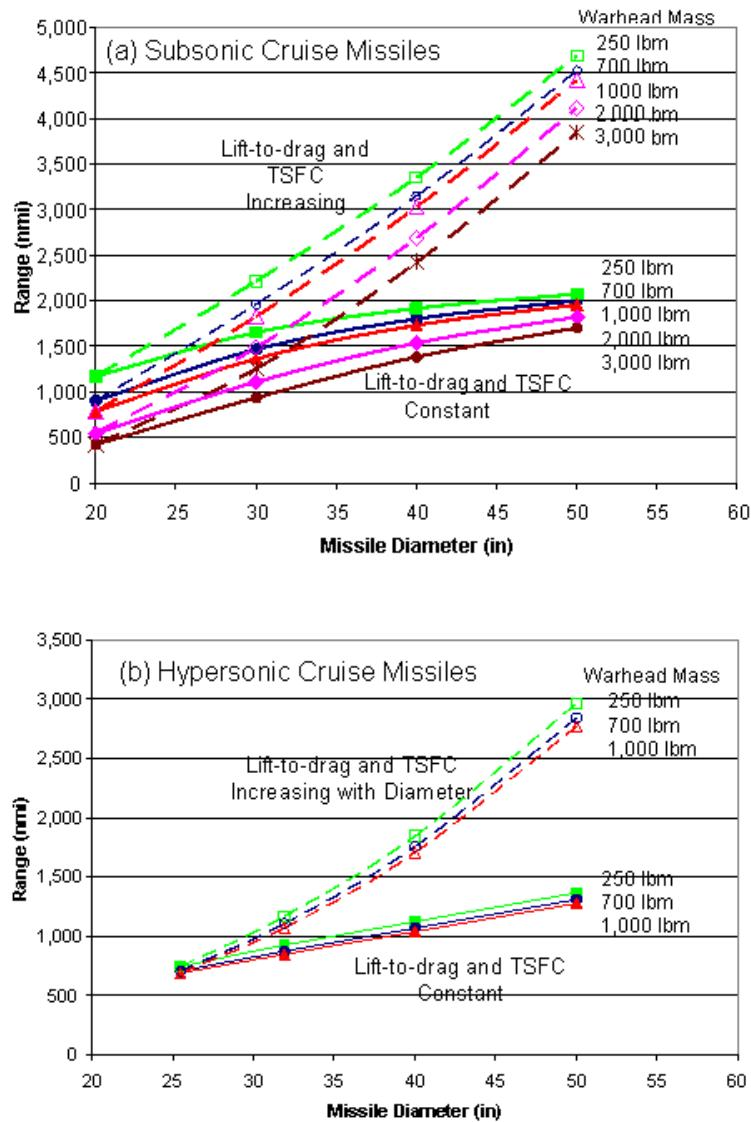
FIGURE 4-14 The impact of missile diameter and payload on range of notional (a) subsonic and (b) hypersonic cruise missiles. The solid curves are based on flight- or laboratory-demonstrated aerodynamic and propulsion technology. The dashed curves illustrate the potential performance improvements that result from potential aerodynamic and propulsion efficiency gains. NOTE: TFSC, thrust specific fuel consumption.
