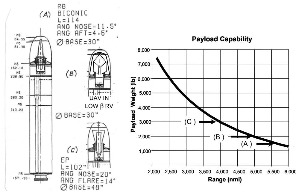
FIGURE 4-10 Candidate configurations for the committee-proposed Conventional Trident Modification (CTM)-2 illustrating concepts for integrating large payloads on a two-stage Trident missile, and results for range versus payload trade-offs for ballistic flight.
